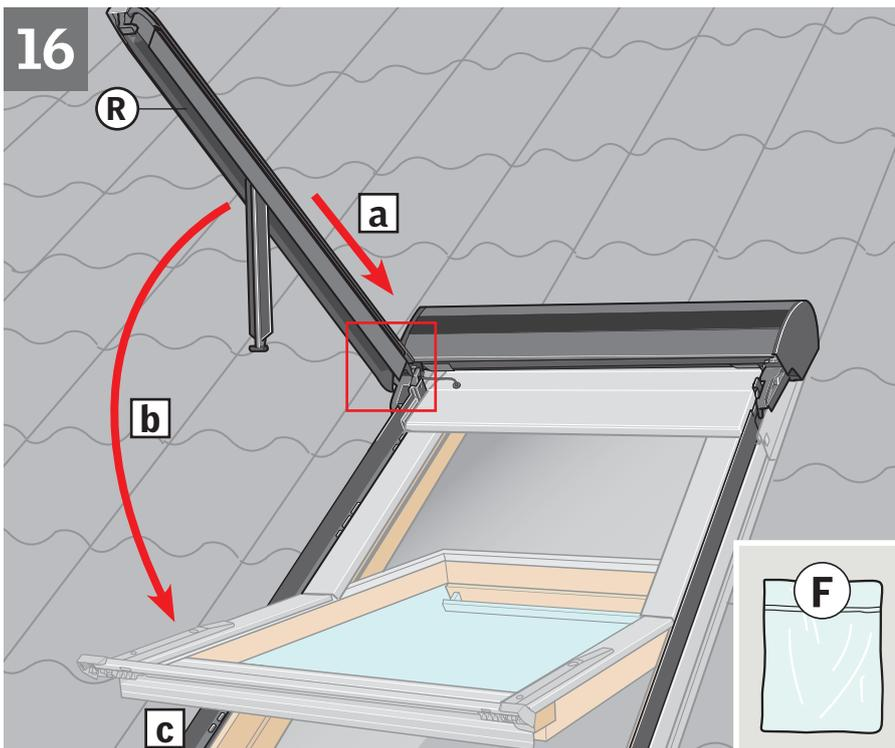
**ENGLISH:** Push side channels into position [a](#) and lay down on side covers [b](#). Attach opening restrictors to side covers with screws [c](#).
