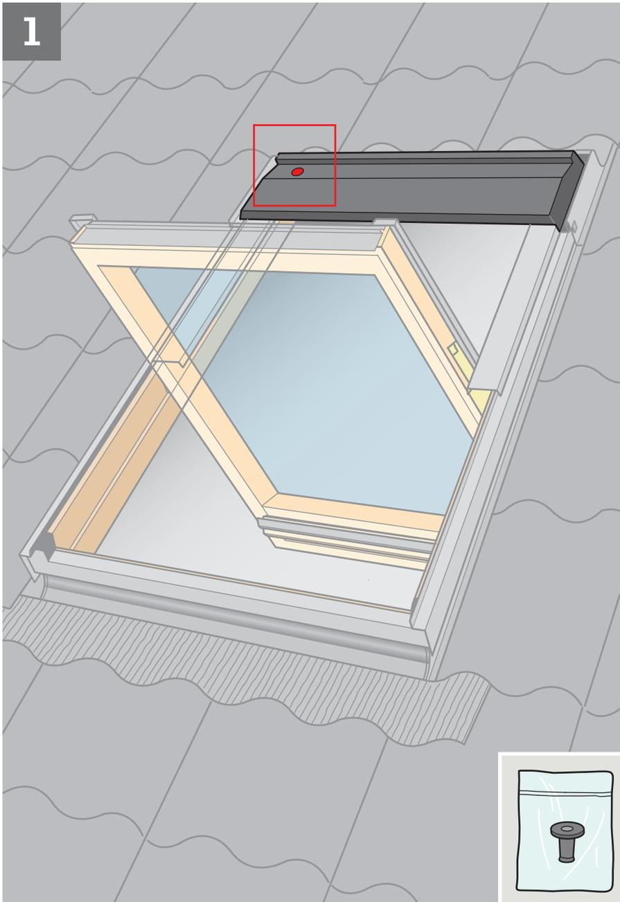
**ENGLISH:** If the window has been fitted with a black screen profile and/or a connection box, remove this/these temporarily [a], [b]. Drill hole [c] and fit rubber grommet [d]. Pull grommet through from the inside [e].
