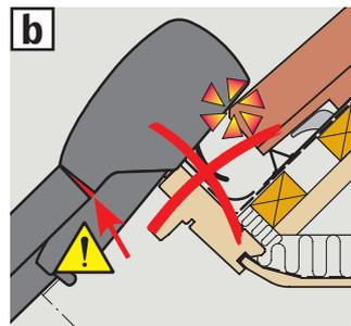
**ENGLISH:** Lower the roller shutter top casing as much as possible. Do **not** press the top casing against the roofing material [a], [b]. Pull cable through hole on window top cover. Fit securing screws after installing the roller shutter top casing [c], [d].
