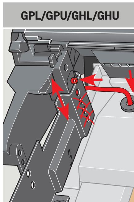
**ENGLISH:** Lower the roller shutter top casing as much as possible. Do **not** press the top casing against the roofing material **[a]**, **[b]**. Pull cable through hole on window top cover.
